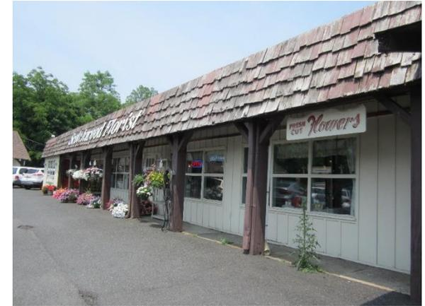
The parking lot is pitched toward the southwest end of the site. The parking spaces at this end can be repaved with porous asphalt to capture stormwater runoff. Roof runoff from the florist shop on the east side of the property can be harvested to water the plants displayed outside the shop by installing a cistern or rain barrel. A preliminary soil assessment suggests that more soil testing would be required before determining the soil's suitability for green infrastructure.
