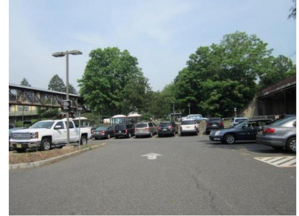
The driveway and parking lot are pitched toward several catch basins draining to local waterways. Parking spaces can be repaved with porous asphalt to promote stormwater infiltration in the parking lots on either side of the train tracks. A preliminary soil assessment suggests that more soil testing would be required before determining the soil's suitability for green infrastructure.
