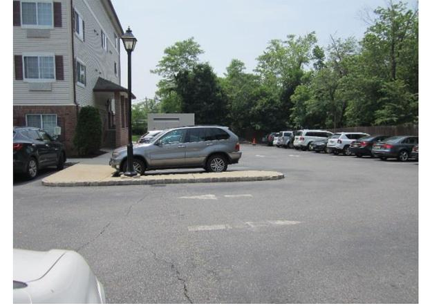
Parking spaces can be repaved with porous asphalt to reduce impervious cover and infiltrate stormwater. A downspout at the east corner of the building can also be disconnected into a cistern to harvest rainwater that the residents can use for watering the existing plants. A preliminary soil assessment suggests that more soil testing would be required before determining the soil's suitability for green infrastructure.
